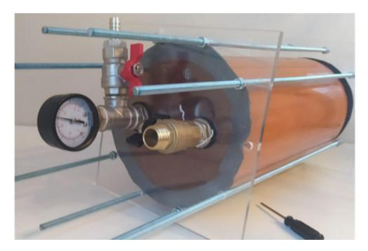
The kit allows you to assemble a simple low pressure test bench with a chamber suitable for placing a CubeSat microsatellite.
